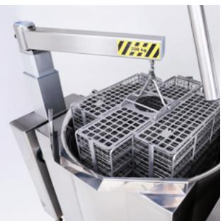
Integrated lifting arm capacity is 200 kg.
