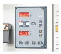
Each chamber is equipped with an independent digital electronic control unit from which baking parameters can be set easily, including:
