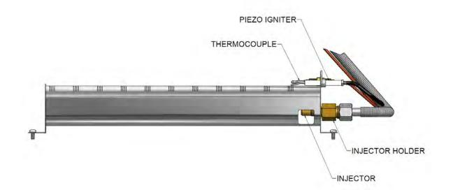
2. Unscrew injector from injector holder and replace with correct size injector as shown in 'Gas Specifications Tables' at rear of this section.
